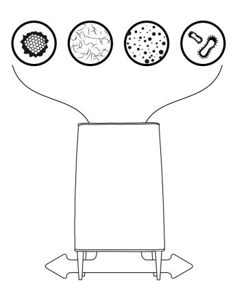
Dirty indoor air is drawn into the top opening of the lampshade and through the filter. The precharged filter captures the particles through a combination of mechanical and electrostatic filtration technologies, ensuring an optimal efficiency for pollen, dust, pet dander, smoke and even bacteria.
